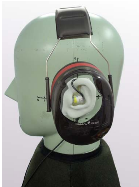
Figure 2 Double ANR protection, cut-away shows personally moulded earplug and position of cable, minimising acoustic leakage.
